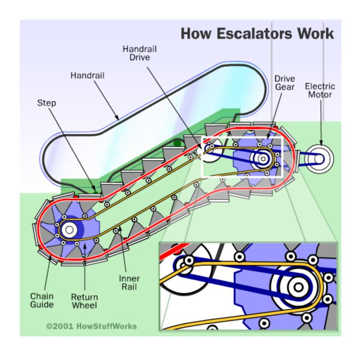
Instead of moving a flat surface, as in a conveyer belt, the chain loops move a series of steps. Therefore, as the chains move, the steps always stay level. At the top and bottom of the escalator, the steps collapse on each other, creating a flat platform. Consequently, this makes it easier to get on and off the escalator. In the diagram, the internal workings of an escalator can be seen.
